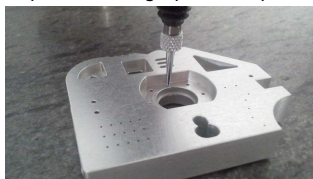
Needle contact-point mounting example
