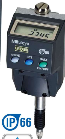
Rated to IP66 water- and dust-proofing standard and oil resistance improved.
