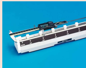
Checking accuracy of caliper (outside measurement)
