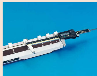
Checking accuracy of caliper (inside measurement)
