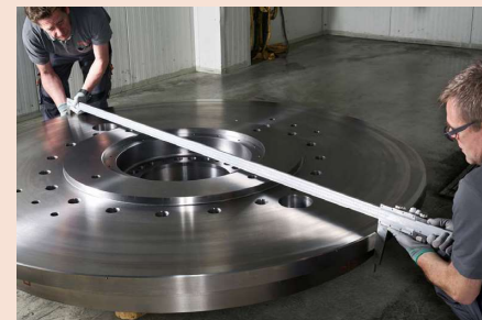
Radiused jaws for accurate ID measurement
