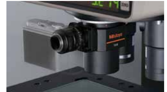
Example of attaching the Projection Lens 10X with C mount on PJ-H30
