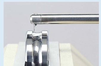
Inner/outer ring contour of a bearing
