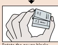
Rotate the gauge blocks while applying slight force to them. You will get a sense of wringing by sliding the blocks.
