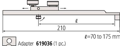
Used for attaching a long gauge block to the base over a stack of regular gauge blocks wrung between the base and long gauge block. The length  $l$  is highly adjustable to accommodate the variable length of the stack.
