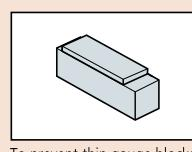
To prevent thin gauge blocks from bending, first wring a thin gauge block onto a thick gauge block.
