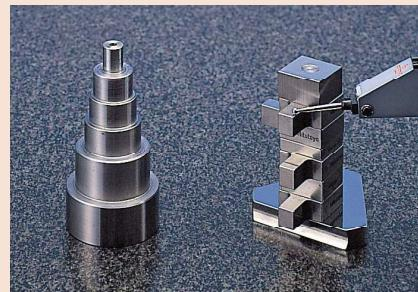
Using plain jaws, gauge blocks, a tie rod and a knurled-head screw a gage was constructed to enable rapid comparison measurement of a stepped workpiece. (Sample workpiece)
