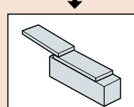
Then, wring the other thin gauge block onto the first thin gauge block.
