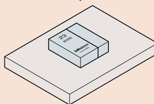
Wipe the exposed measuring face (s) and continue building up the stack, in the same manner as above, until complete.
