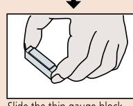
Slide the thin gauge block while pressing the entire overlapped area to align the measuring faces with each other.
