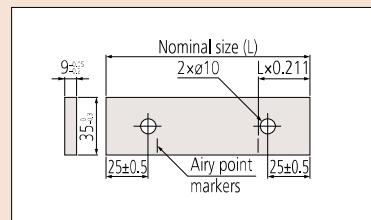
Two coupling holes are provided in this type of block for the purpose of joining two long blocks together and/or attaching accessories using special connectors. (See page E-19 for connector types available.)
