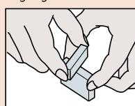
Cross the gauge blocks at 90° in the middle of the measuring faces.
