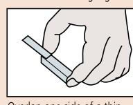
Overlap one side of a thin gauge block on one side of a thick gauge block.
