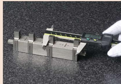
Using plain jaws, gauge blocks, a tie rod and a knurled-head screw a gage was constructed to enable rapid checking of the accuracy of a caliper at selected points.
