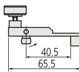
Used for attaching a long gauge block directly to the base.
