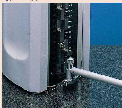
Bore gage zero-setting
