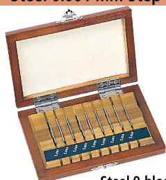
Steel 9-block set (1.001 to 1.009 mm)
