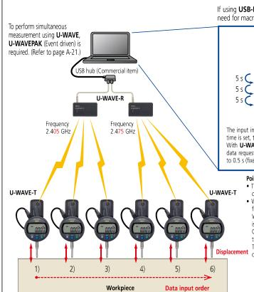
Automatically obtains displacement data in a certain input interval
