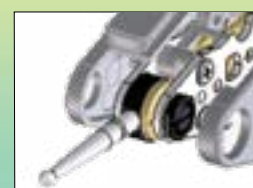
Stylus bearing screw held in sub-plate.
