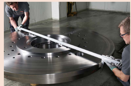
Radiused jaws for accurate ID measurement
