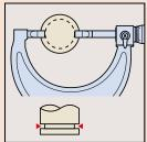
For inside diameter, and narrow groove measurement
