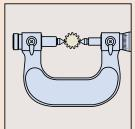
Measurement of gear over-pin
