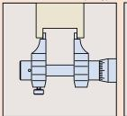
Inside micrometer, caliper type
