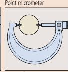
For pipe thickness measurement For root diameter measurement
