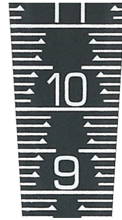
Stepped millimeter graduation prevents misreading
